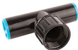
6821304 6822304(MASTER PAK) (40/PK) 1/2" riser swivel tee fits 0.704" to 0.710" OD tubing
