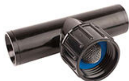
6821308 6822308(MASTER PAK) (15/PK) 3/4" FHT swivel tee w/screen fits 0.680" to 0.704" OD tubing
