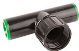
6821302 6822302(MASTER PAK) (40/PK) 1/2" riser swivel tee fits 0.610" to 0.630" OD tubing
