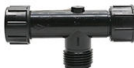
6821370 3/4" Plastic Filter Tee, stainless steel 150 mesh (3/4" swivel inlet x 3/4" MHT outlet) (max flow of 10 gpm)
